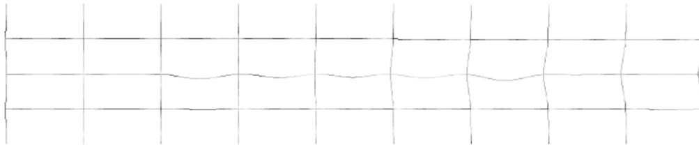
Fig. 13. The deformed shape of the two-dimensional frame structure under spreading fire
