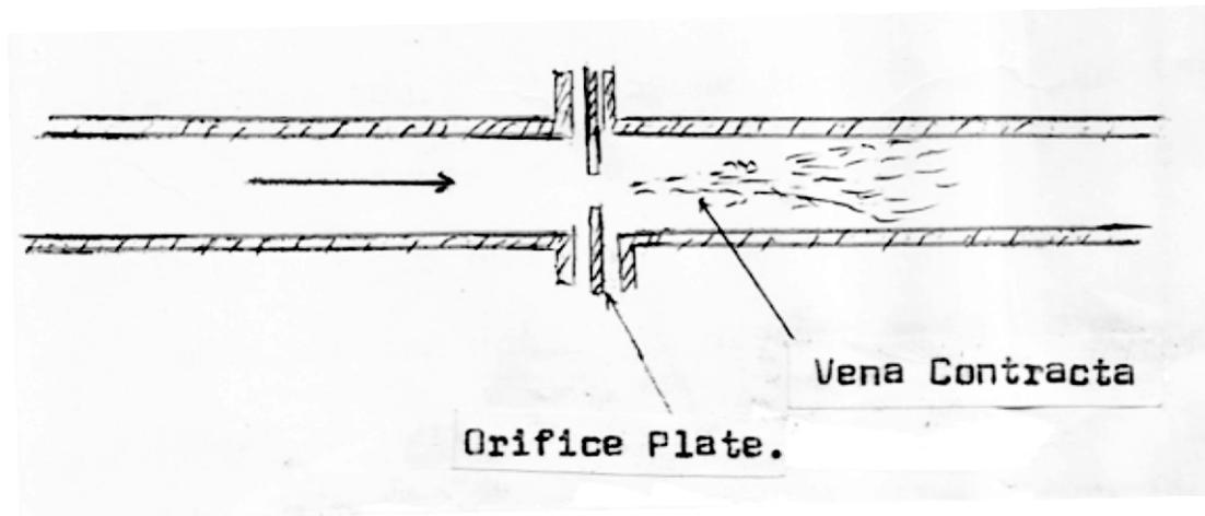
Hughes (1974) suggested that the orifices can be used very selectively to constrain peak demand only in those sections of a system that would otherwise be in danger of experiencing negative pressures during peak demand periods. The advantages of the system are (Osanebi, 1985)
