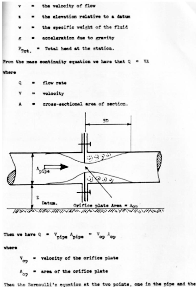
Fig. 2: Plain Type Orifice Plate
