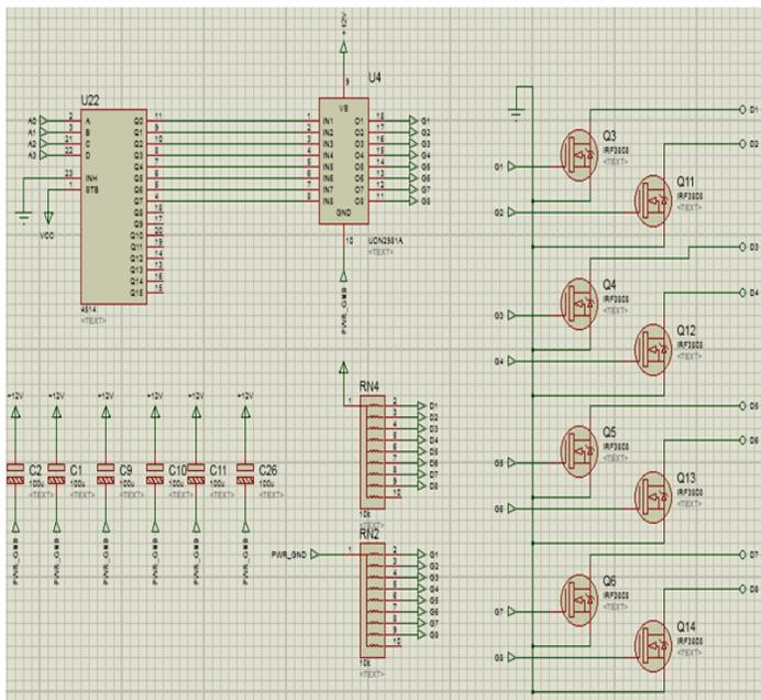
Figure 3 Schematic for Row Driver
