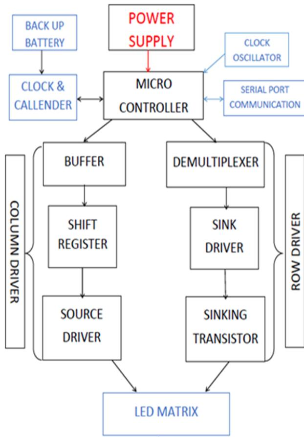
Figure 1 Block diagram of the circuit
