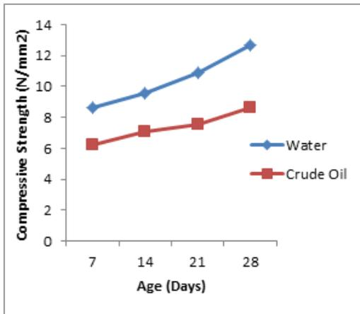
Figure 5: Rate of Development of Compressive Strength of Concrete for 1:3:6 Mix Design
