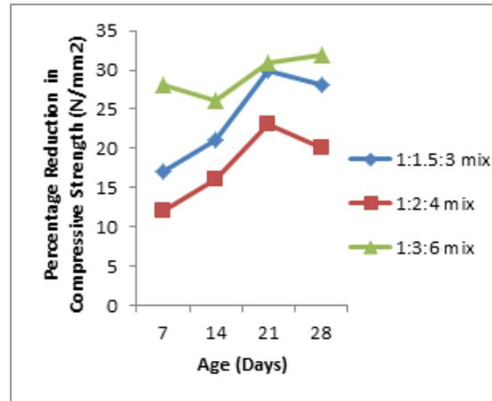
Figure 6: Percentage Reduction of Compressive Strength for the different mix ratios
