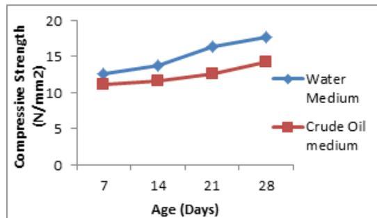
Figure 4: Rate of Development of Compressive Strength of Concrete for 1:1.5:3 Mix Design
