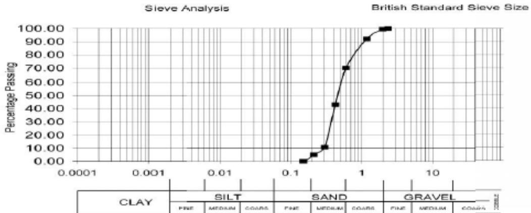
Figure 1: Grading Curve of Fine Aggregate
