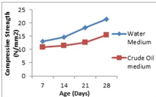
Figure 3: Rate of Development of Compressive Strength of Concrete for 1:2:4 Mix Design
