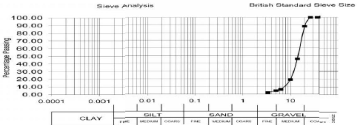
Figure 2. Grading Curve of Coarse Aggregate
