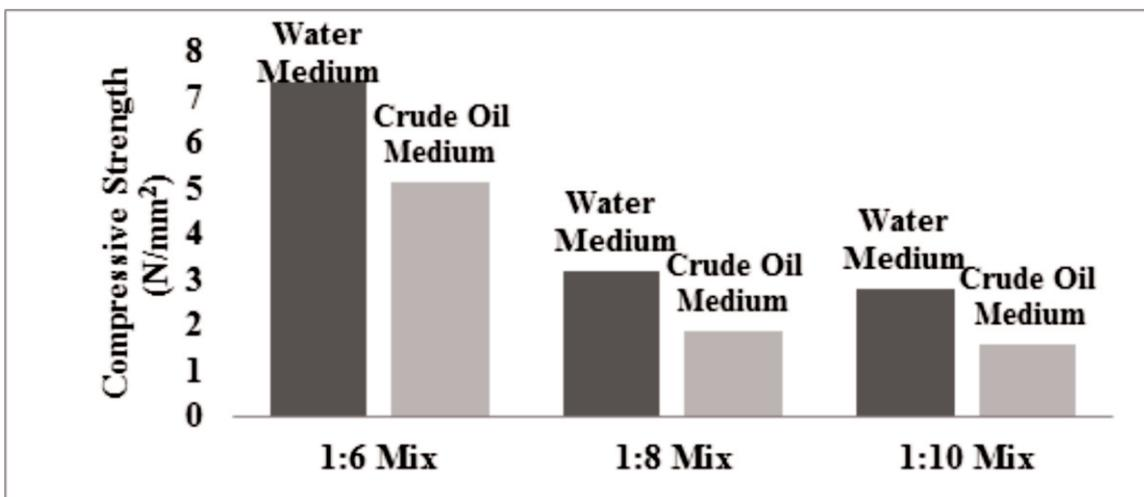
Figure 7: Average Compressive Strength of Sandcrete for both curing media and the three mixes Considered at 42days
