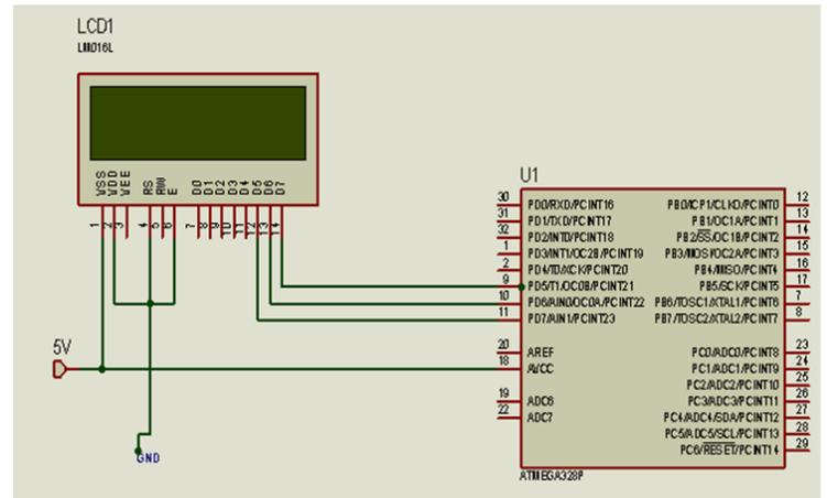
Figure 7: LCD interfaced with ATmega16
