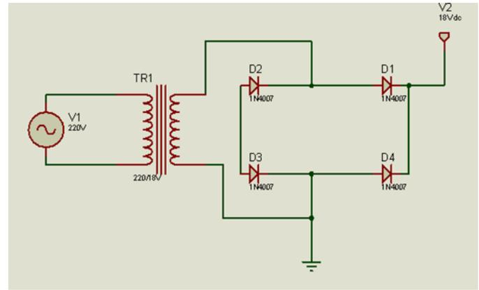
Figure 2 Power Supply Circuit
