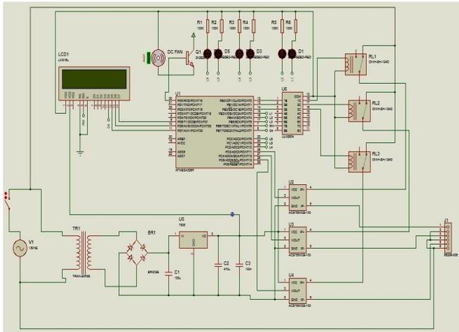
Figure 8 Complete circuit diagram of the overload detection system
