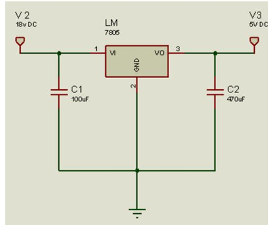
Figure 3 Voltage regulator circuit
