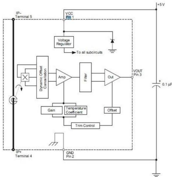
Figure 4: Functional block diagram of ACS755 current sensor
