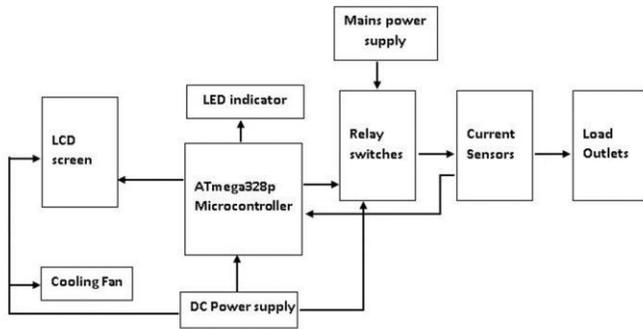
Figure 1 Block diagram of the Overload detection system
