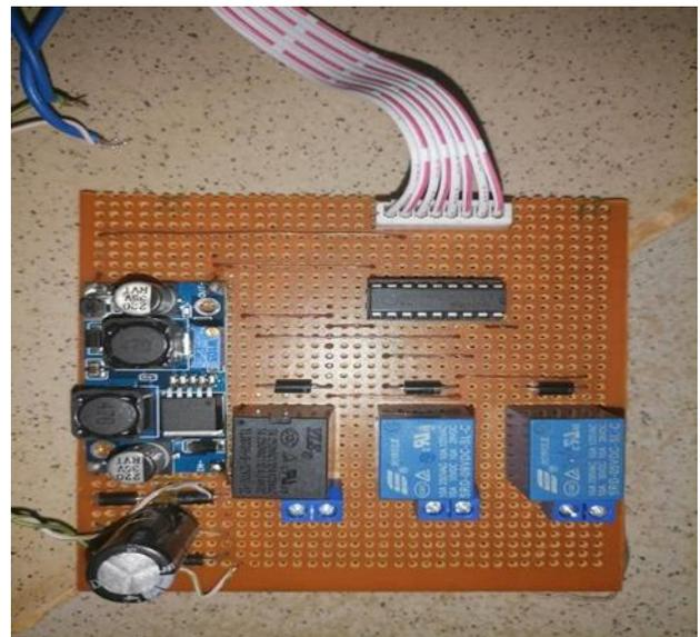
Figure 9 Relay Module
