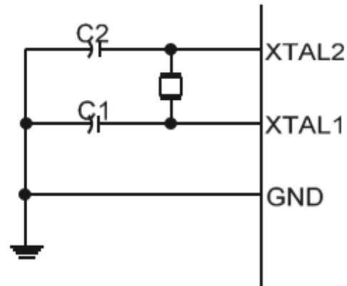
Figure 5 Crystal oscillator connection to ATMEGA328P
