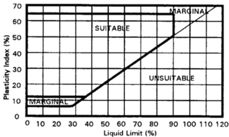
Figure 3: Plasticity and Suitability Criteria of Material for Landfill Liners. Source: (Jones et al., 1995)
