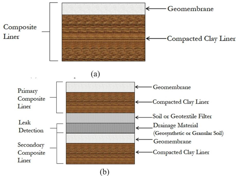
Figure 1: Variant of Compacted Clay Liner used in Sanitary Landfill. Where (a) Single Compacted Liner and (b): double compacted Liners. Source: (Koerne and Daniel, 1997)
