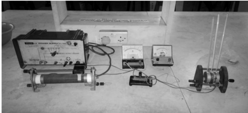
Fig 2: Experimental set up of the Lee's disc method
