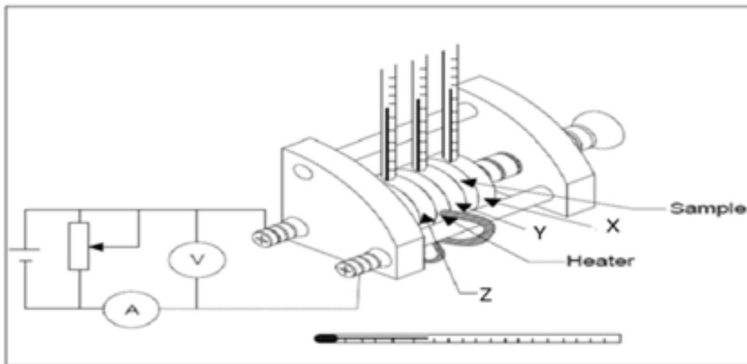
*Fig 1: Schematic set-up of lee's disc experiment (Oluyamo et al., 2012).*
