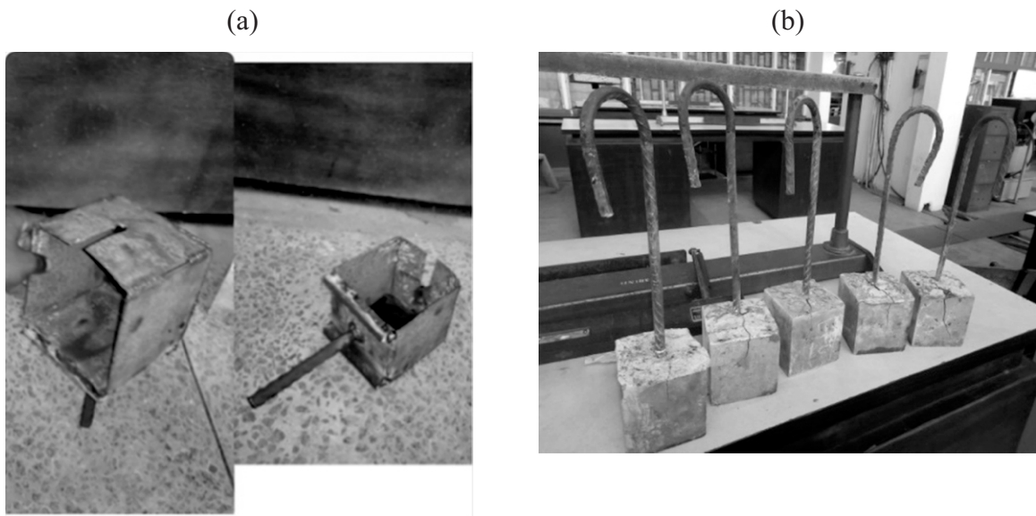
Figure 2: (a) Concrete bracket for holding concrete cubes (b) concrete cubes after testing showing cracks at interface between concrete and rebar
