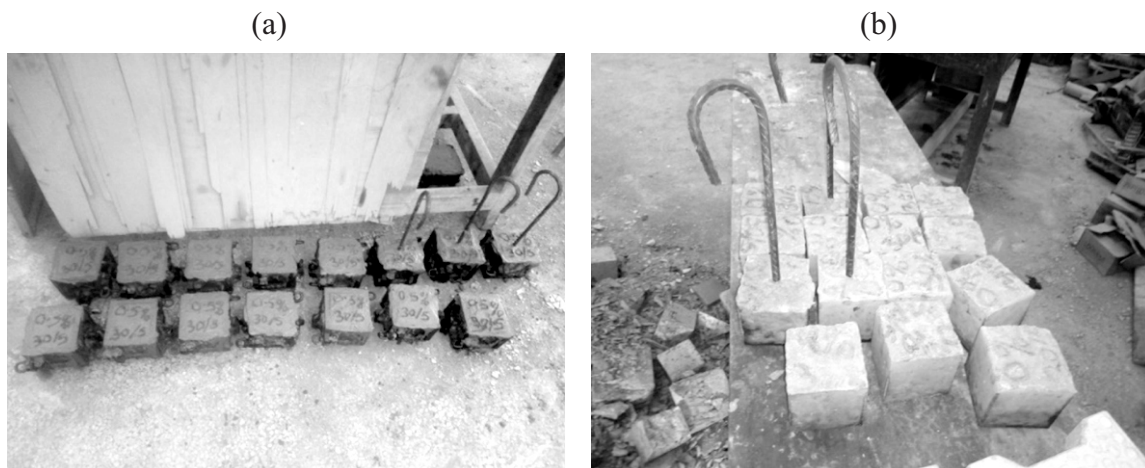
Figure 1: (a) Concrete cubes left to cure under air for 24 hours (b) Concrete cubes after de-moulding
