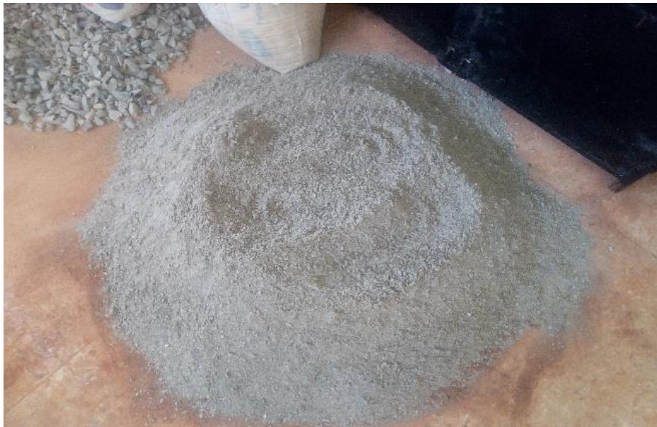
Figure 1: Quarry dust sample
