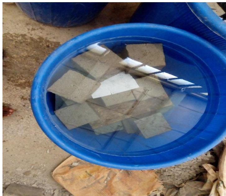
Figure 4: cubes in Curing Tank.
