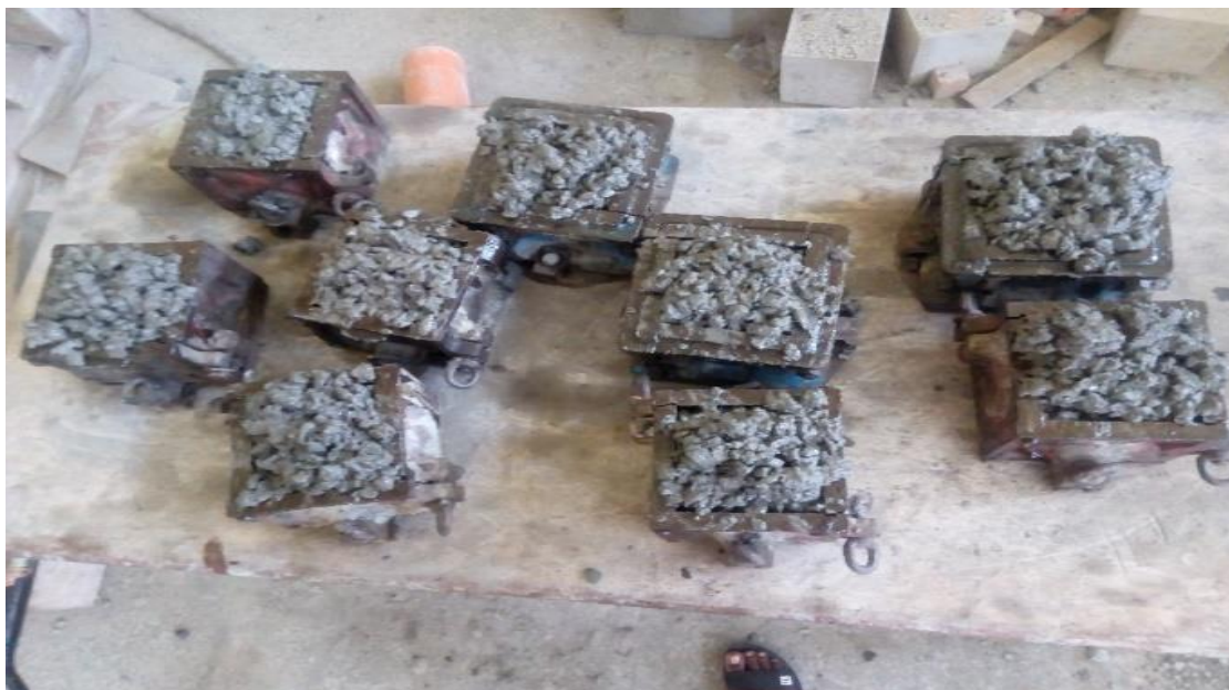
Figure 2: Concrete in cubes moulds
