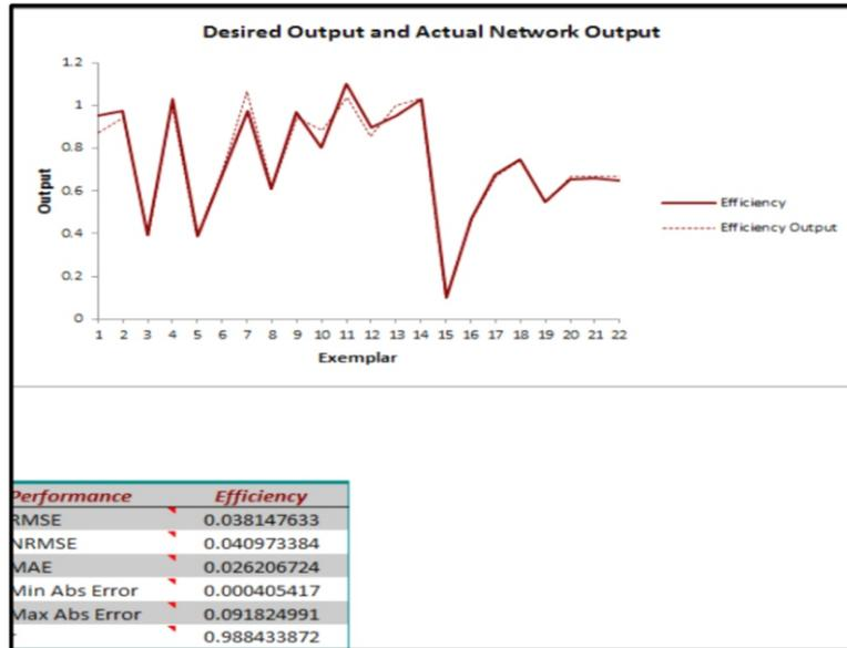
Figure 5: predicted versus observed sorption efficiency of Pb(II) ion using MNN
