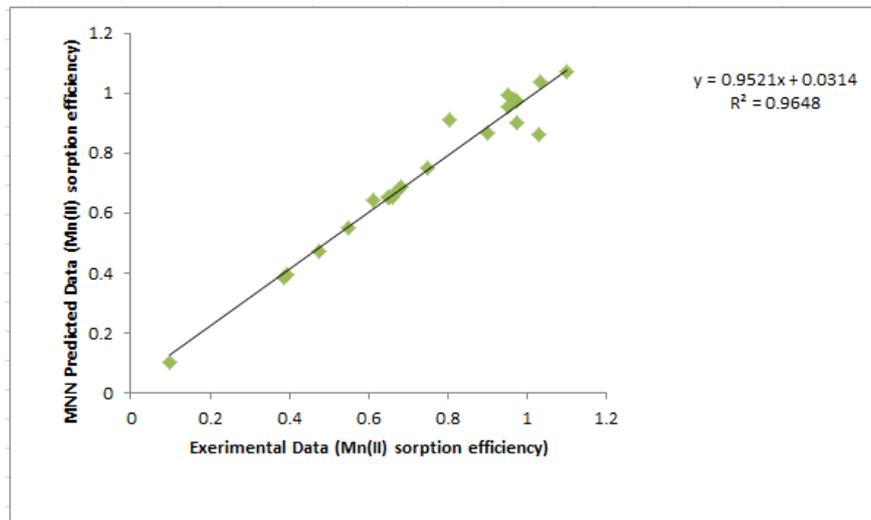
Figure : Performance of MNN on new input data
